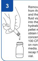
Remove the cap from the pellet vial and the hydrating fluid vial. Tip 1 pellet into the 1.2 ml vial of hydrating fluid. Only 1 pellet must be used to obtain the challenge concentration of 10-100 CFU per 0.1 ml on non-selective media. Immediately recap hydrating fluid
