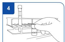
Immediately recap the vial with the hydrated material and place into a 34°C-38°C incubator for 30 minutes to ensure complete hydration.
