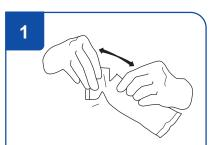
Allow the unopened KWIK-STIK™ pouch to equilibrate to room temperature. Tear open pouch at notch and remove the KWIK-STIK unit.
