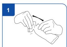
Allow the unopened Lab-Elite™ (KWIK-STIK™) pouch to equilibrate to room temperature. Tear open pouch at notch and remove the KWIK-STIK unit.
