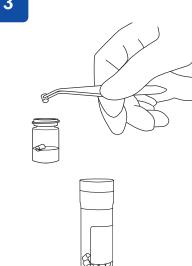
With a sterile forceps, transfer 2 pellets into the 2 ml vial of hydrating fluid. Do not remove the desiccant from vial. Two pellets must be used to obtain the challenge concentration of 10–100 CFU per 0.1 ml on non-selective media. Immediately stopper and recap the pellet vial and return the remaining lyophilized material to refrigerated storage 2°C–8°C.
