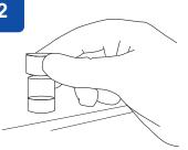
While the pellets are equilibrating, prewarm the hydrating fluid to 34°C–38°C (at least 30 minutes).
