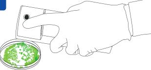
Hold the lamp over the microorganism culture being tested for fluorescence. Visually examine the culture and determine whether or not it fluoresces. The expected result when the culture is being grown on Tryptic Soy Agar is a green fluorescence. Other agars and variables within each laboraory's processes may produce fluorescence with varying colors, or may mask the expression of the GFP due to biochemical byproducts produced during the test.
