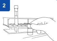
While the pellets are equilibrating, prewarm the hydrating fluid vial and a tube of 9.0 ml of phosphate buffer pH 7.2 to 34°C-38°C (at least 30 minutes).
