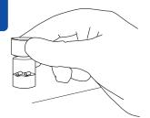
Immediately recap the vial with the hydrated material and place into a 34°C–38°C incubator for 30 minutes to ensure complete hydration.
